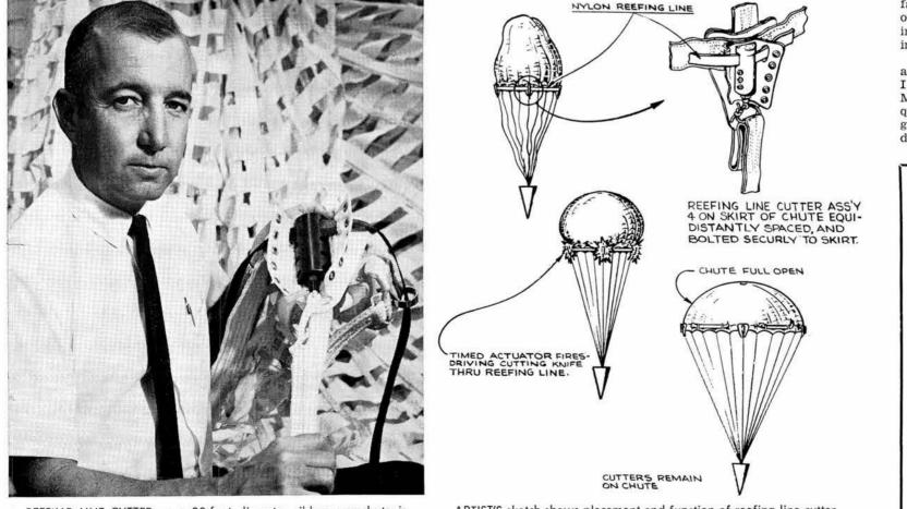
REEFING LINE CUTTER on a 20-foot diameter ribbon parachute is displayed by James P. Gallagher (9323), inventor of the device.
